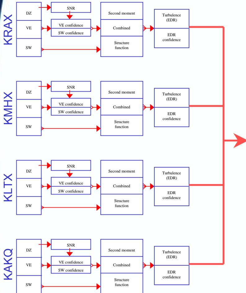
Distance\* - and confidence-weighted mean EDR on grid<sup>†</sup>
