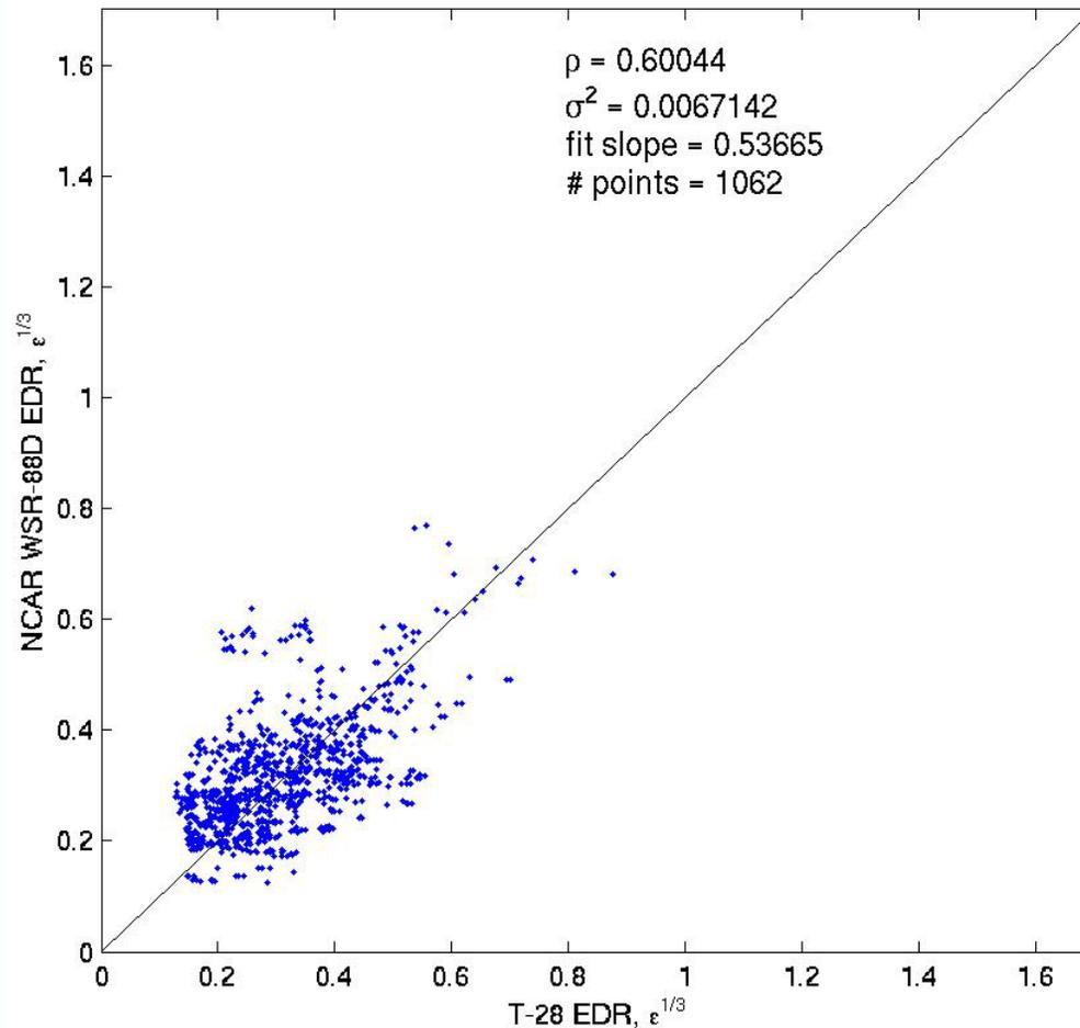
NTDA “combined” method EDR with more extensive QC (1 km disc median) vs. *in situ* EDR, all STEPS flights
