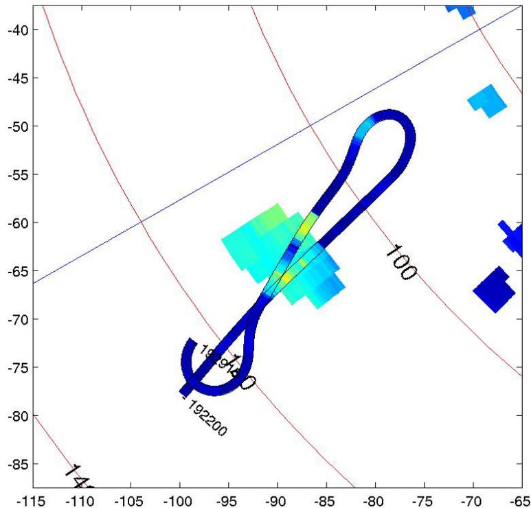
B-757 EDR (0 to 0.7  $m^{2/3}/s$ ) from 15 April 2004, 19:22–19:29 overlaid on 19:26 KLTIX 2.4° NTDA EDR (refl. between 5-30 dBZ)
