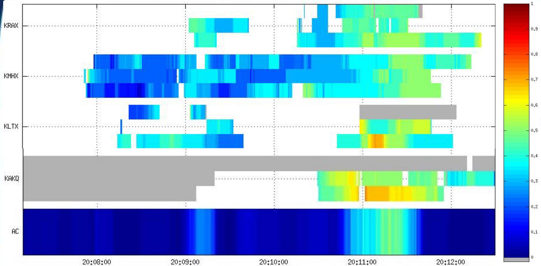
NASA B-757 aircraft EDR timeseries (bottom) and 2-km disc median NTDA EDRs (0 to 1  $\text{m}^{2/3}/\text{s}$ ) along aircraft track from nearest 3 sweeps of multiple NEXRADs, 15 April 2002
