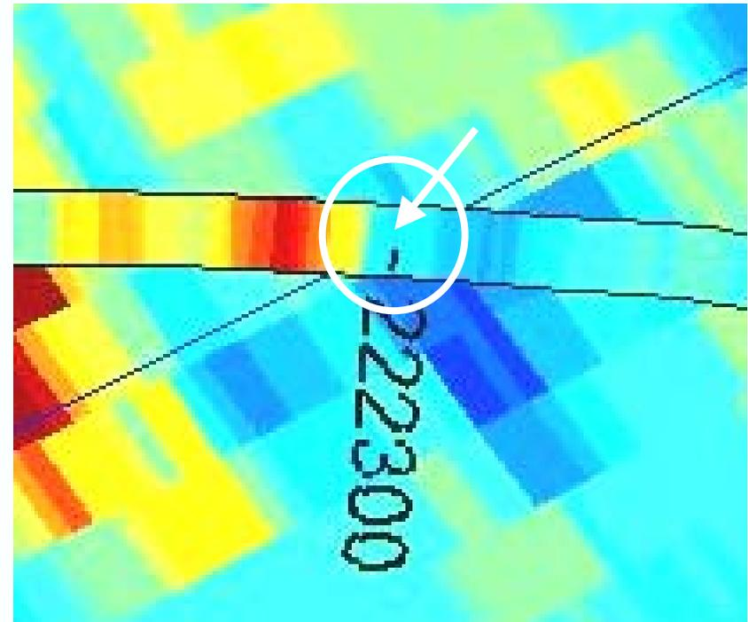
Example: The *in situ* EDR at 22:30 is compared to the median of radar values in a 1-km disc surrounding its location projected onto the nearest sweep
