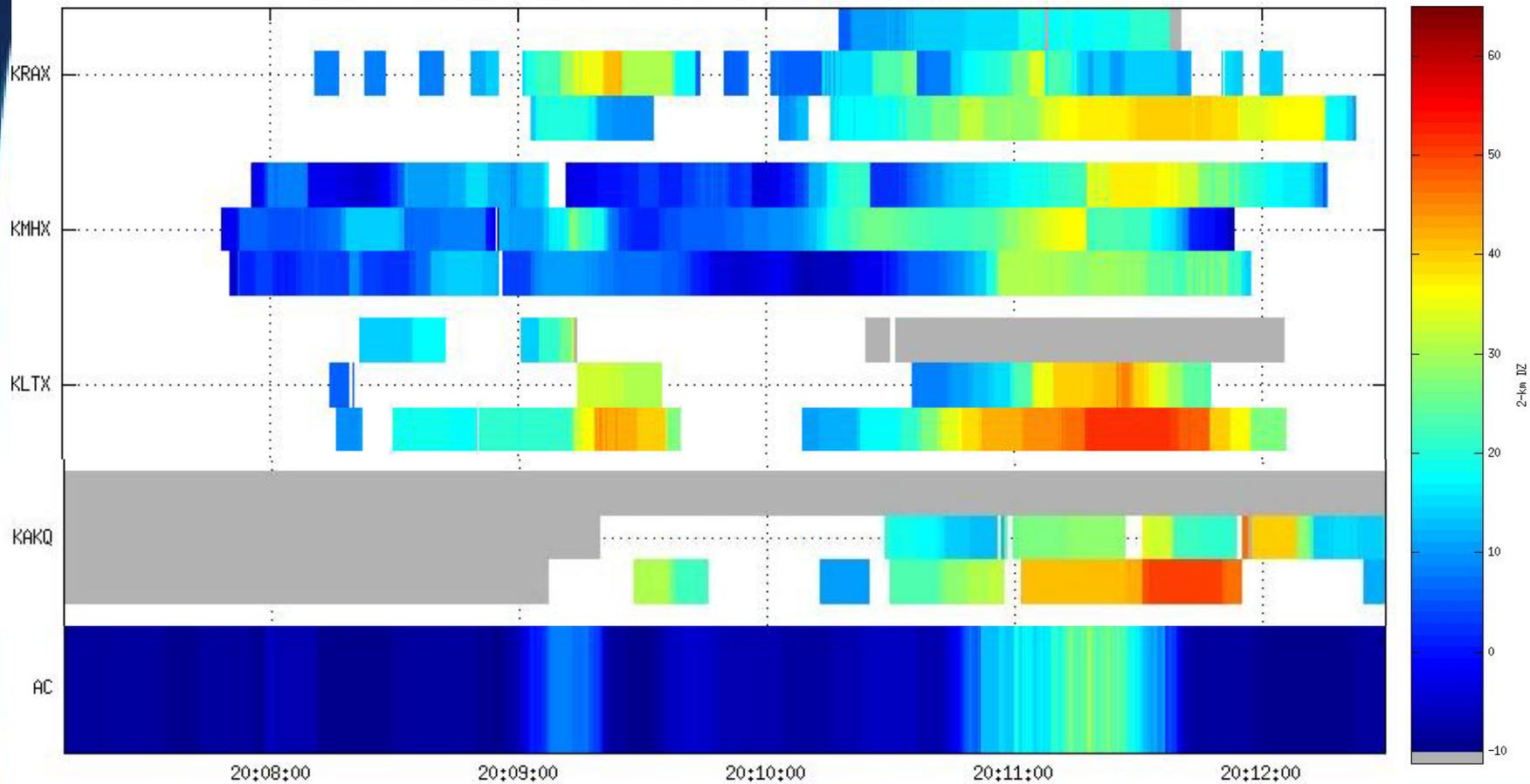
NASA B-757 aircraft EDR timeseries (0 to 1  $\text{m}^{2/3}/\text{s}$ , bottom) and 2-km disc median radar reflectivity (-10 to 65 dBZ) along aircraft track from nearest 3 sweeps of multiple NEXRADs, 15 April 2002
