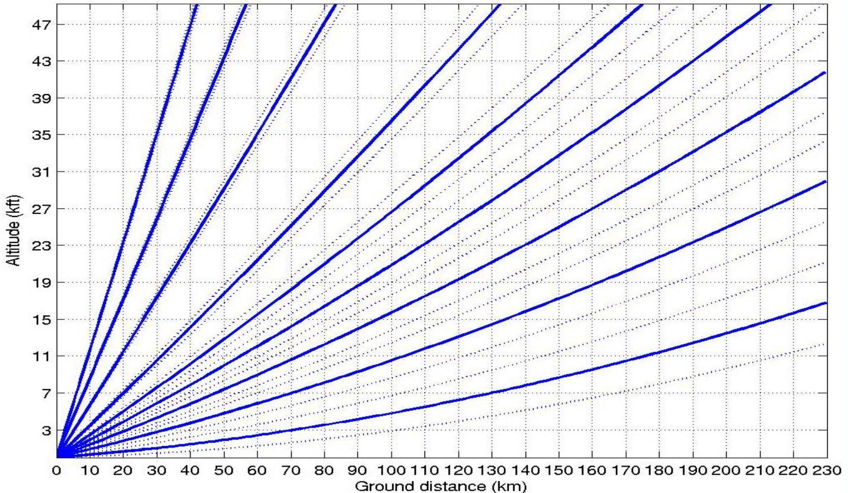
Altitude above radar for 0.5, 1.5, 2.4, 3.3, 4.3, 6.0, 9.9, 14.6, and 19.5° tilts as a function of ground distance. Dotted lines represent  $\pm 1/3^\circ$  beam paths.
