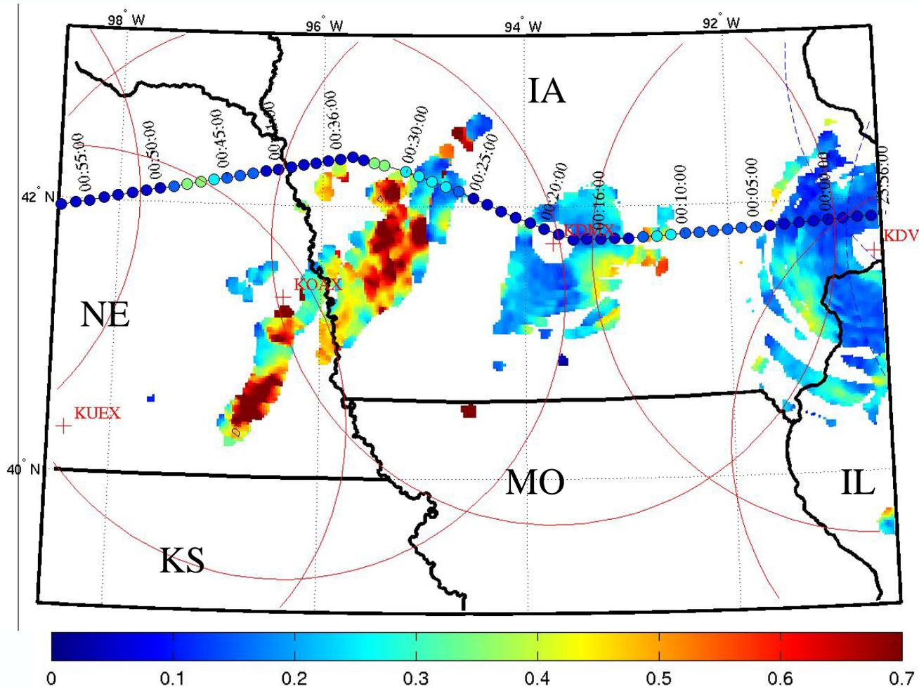
Merged NEXRAD NTDA EDRs and overlaid *in situ* EDRs ,  $m^{2/3}/s$
