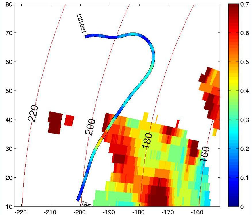
B-757 EDR (0 to 0.7  $m^{2/3}/s$ ) from 30 April 2004, 18:55–19:01 overlaid on KFFC 2.4° NTDA EDR (refl. between 5-15 dBZ)
